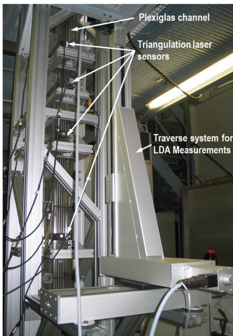
Figure 3: Test section of the “ALAIN” test loop with measurement systems
