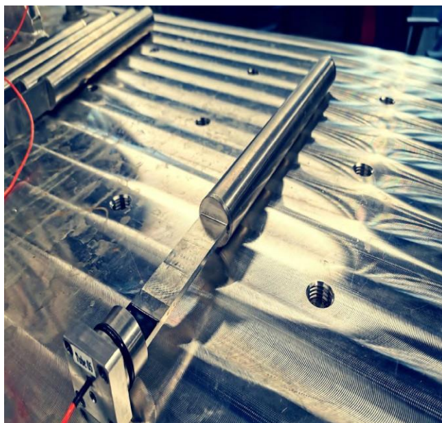
Figure 3. The experimental rig: TITAN. Tube instrumented with a flexible blade.
